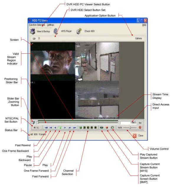
Fig.1. DVR HDD PC Viewer User Interface
